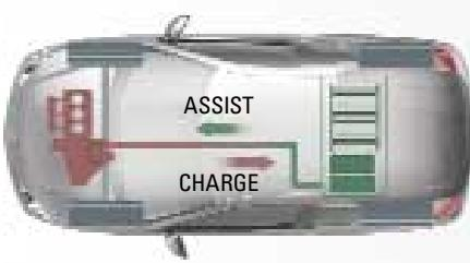
*The Insight's Integrated Motor Assist (IMA) system uses a lean-burn 1.0 liter VTEC-E engine assisted by a compact, electric motor.*
