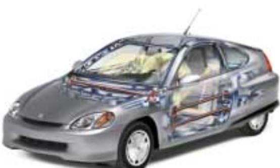
*Crumple Zones built into the Insight's highly rigid aluminum body are designed to help protect the driver and passenger in an impact.*
